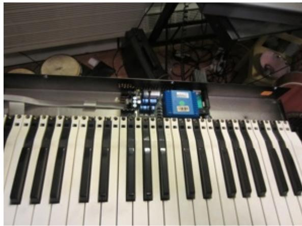
I realized at this point that I was going to have to take the whole keybed apart from the bottom black metal frame. This is done by removed those 12 or so screws on the bottom.
