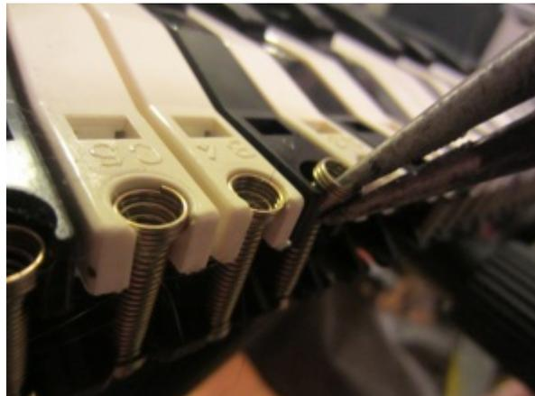
To remove a key, remove the spring, then gently pull up and you will feel it click letting go. Then pull it forward and away. Replacing is the reverse of this. But, to fix the key contact, this is all unnecessary.
