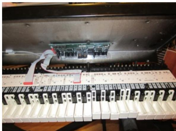
Removing those two ribbon cables allows you to set aside the black metal bottom, leaving only the keybed. Here are some pics of the keybed, and some of the keys themselves. It turns
